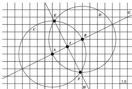
The picture shows one possible instance for  $A = (1, 1)$  and  $B = (5, 3)$ . In this GSP points  $E$  and  $F$  have the same definition, namely being the intersection of the two circles. Only for the “right” choices you will obtain an actual instance of the GSP in which the final point is indeed the midpoint of  $A$  and  $B$ .
